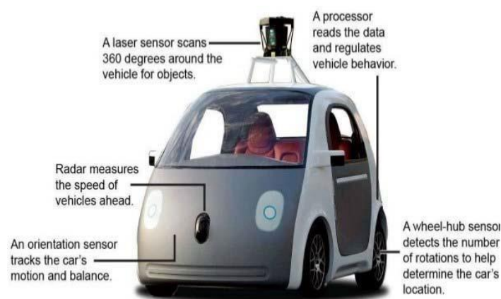
Figure. Basic sensors of Google's driverless car.
